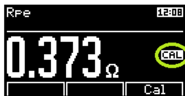
Figure 46: Incorrect compensation for the test leads
