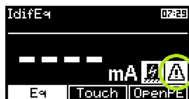
Figure 35: Warning concerning of a point of danger
