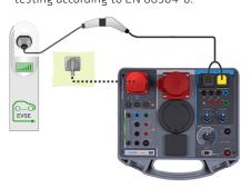
Simulation of faults on mains for verification of Mode 2 electrical vehicle (EV) charging cable safety features.
