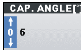
Figure 28: Current leads voltage by 5^\circ angle
