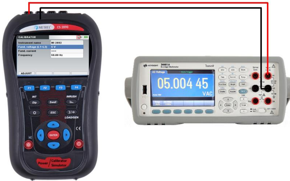
Figure 13: Connection for the voltage adjustment procedure using substandard Volt-meter
