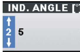
Figure 27: Current lags voltage by 25^\circ angle
