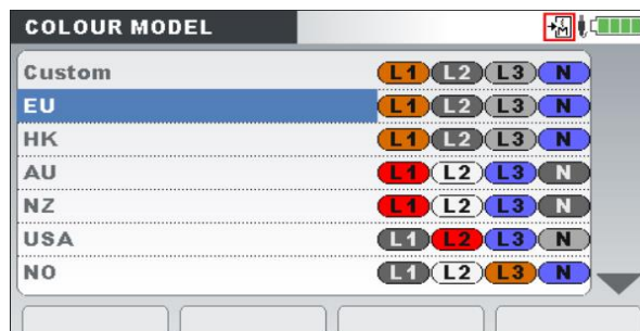
Figure 7: Colour representation of phase voltages
