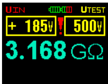
Fig. 3.7a Example of RISO measurement result (discharging in progress)
