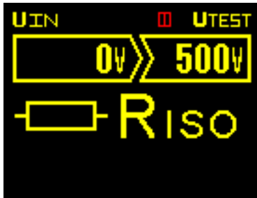
Fig. 3.2a Indication of low battery
