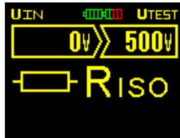
Fig. 3.5 Example of setting for insulation resistance measurement
