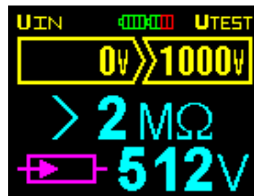
Fig. 3.8b Example of a measurement result (a GDT is connected in the measured circuit)
