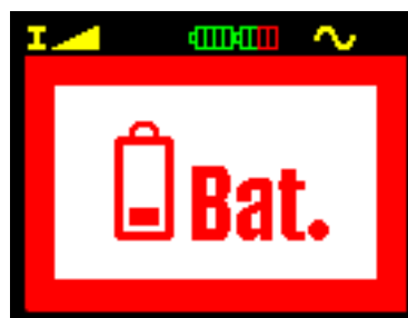
Fig. 3.6b Low battery after the START key was pressed
