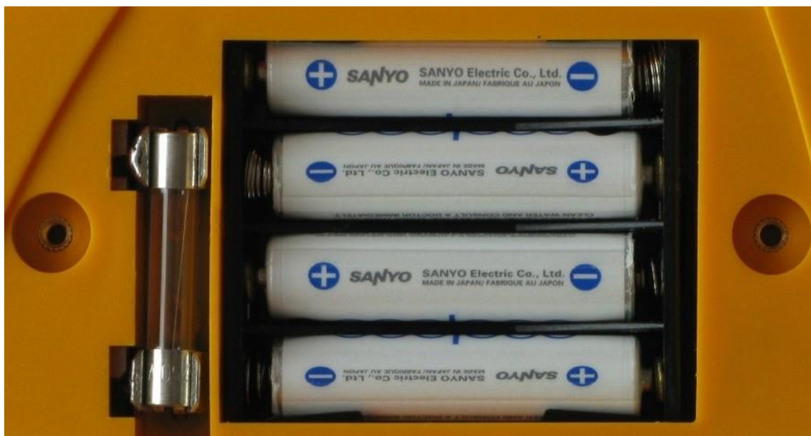
Fig. 4.1 Correct batteries/accumulators polarity and the fuse location
