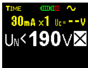
Fig. 3.11 Example of settings for trip-out time measurement
