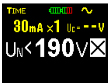
Fig. 3.16a Phase voltage not present on the test tip
