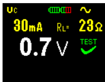
Fig. 3.10 Example of contact voltage measurement result
