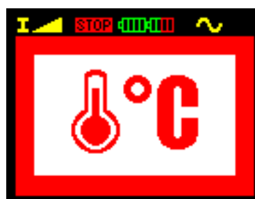
Fig. 3.7b High temperature after the START key is pressed
