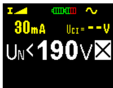
Fig. 3.14 Example of settings for trip-out current measurement
