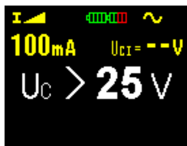
Fig. 3.4b Contact voltage > 25 V
