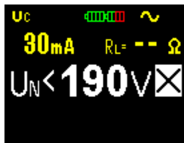
Fig. 3.8 Example of settings for contact voltage measurement
