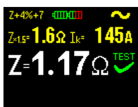
Fig. 3.13 Example of Loop/Line resistance result which takes into account the measurement error
