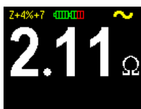
Fig. 3.11 Example of Loop/Line resistance result which takes into account the measurement error
