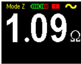
Fig. 3.5a Indication of high temp. (Basic display mode, example)
