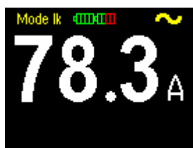
Fig. 3.9 Example of prospective fault/short-circuit current
