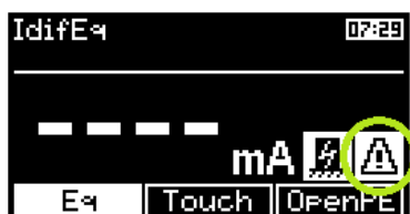
Figure 35: Warning concerning of a point of danger
