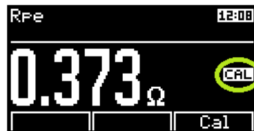
Figure 46: Incorrect compensation for the test leads
