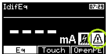
Figure 35: Warning concerning of a point of danger
