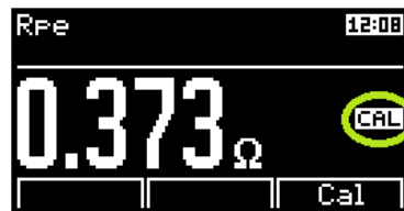
Figure 46: Incorrect compensation for the test leads
