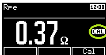
Figure 28: Incorrect compensation for the test leads
