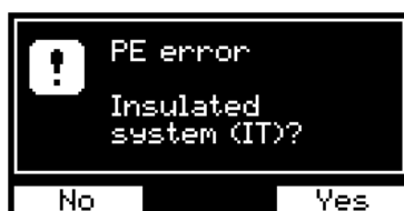
Figure 5: Warning message: PE error (IT systems)
