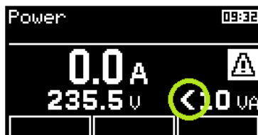
Figure 26: Measured value is out of range (min)
