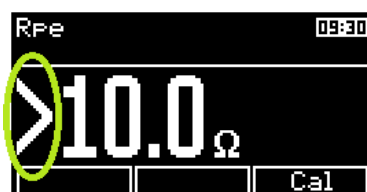
Figure 25: Measured value is out of range (max)
