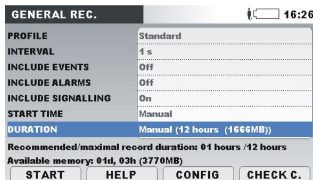
Figure 7.1: General Recorder setup to allow auto-recording restart, when reaches maximum file length
