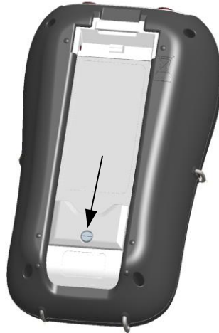
Figure 8.2: Closing the battery compartment cover
