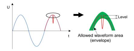
Figure 176: Transients trigger detection (envelope)
