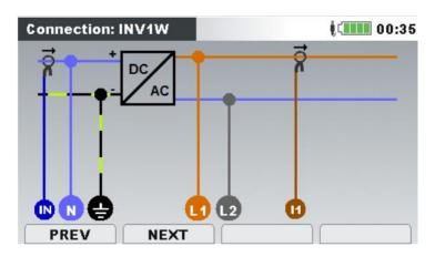
Figure 118: Choosing single- phase Inverter system on instrument
