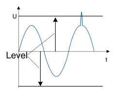
Figure 177: Transients trigger detection (level)
