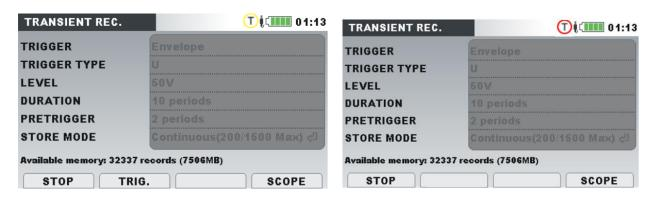
Figure 66: Transient recorder capture screen (waiting phase/recording) - MI 2892/MI 2885
