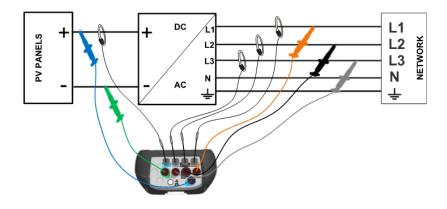
Figure 121: Three – phase inverter system
