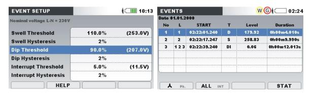
Figure 162:Voltage dip related screens on the instrument
