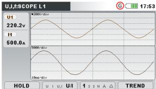
Figure 21: Voltage and current waveform (single mode)
