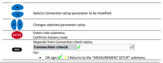
• Fail sign ( ) enter into "CONNECTION CHECK" submenu. It is expected that user will resolve this issue before continuing with measurements.
