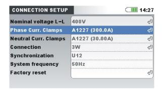
Figure 132: Automatically recognised clamps setup
