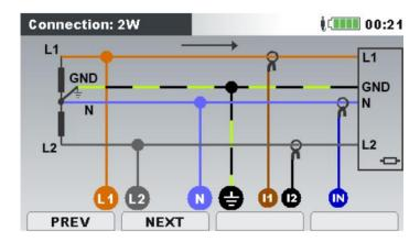
Figure 116: Choosing 2-phase 4-wire system on instrument
