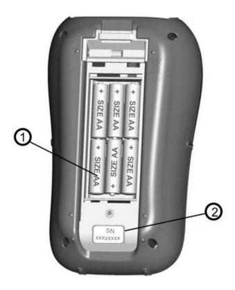
Figure 181: Battery compartment
