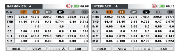
Figure 39: Harmonics and inter-harmonics (METER) screens
