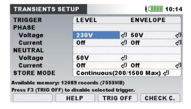
Figure 63: Transient recorder setup screen – MI 2893
