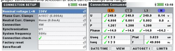
Figure 76: PQI setup connection and Connection check
