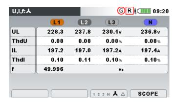
Figure 85: U,I,f meter screen in recalled snapshot record
