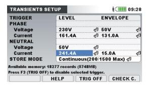
Figure 94: Transient setup screen - MI 2893
