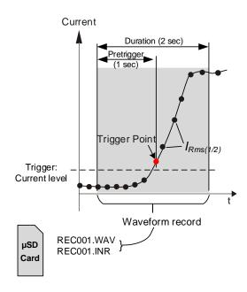
Figure 172: Current Level Triggering (Inrush)
