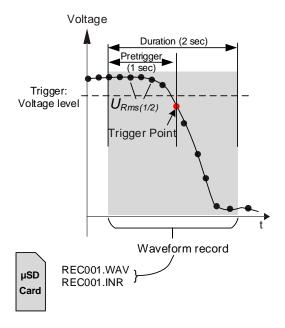
Figure 171: Voltage Level Triggering
