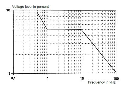
Figure 178: Mains signalling voltage level limits according to EN50160
