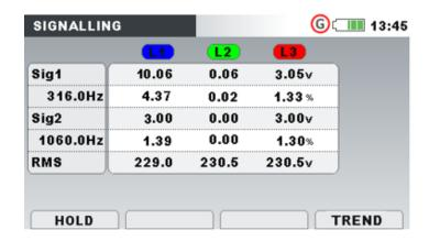
Figure 53: Signalling meter screen
