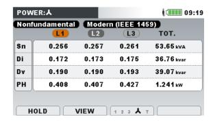
Figure 30: Power measurements summary (nonfundamental)
