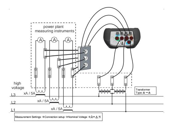
Figure 123: Connecting instrument to the existing current transformers in medium voltage system (Aaron / OpenDelta)
