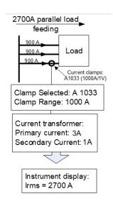
Figure 129: Parallel feeding of large load
