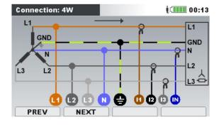
Figure 108: Choosing 3-phase 4-wire system on instrument
