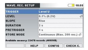
Figure 58: Waveform recorder setup screen
