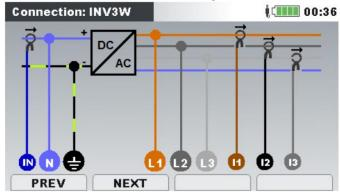
Figure 120: Choosing three- phase Inverter system on instrument
