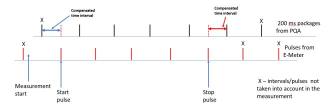
Figure 75: E - Meter measuring accuracy comparison methods
