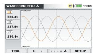
Figure 61: Waveform recorder scope screen
