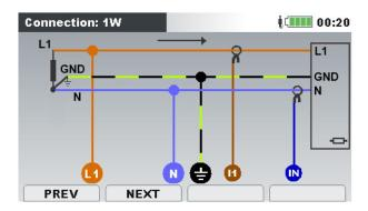
Figure 114: Choosing 1-phase 3-wire system on instrument
