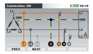
Figure 110: Choosing 3-phase 3-wire system on instrument
