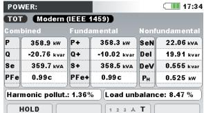
Figure 32: Detailed power measurements at phase L1
