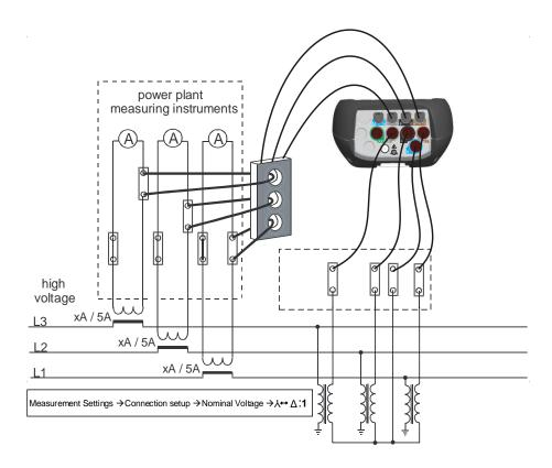
Figure 126: Connecting instrument to the existing current transformers in medium voltage system (Star – Star)
