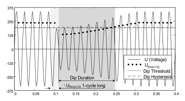
Figure 160:U<sub>Rms(1/2)</sub> 1-cycle measurement
