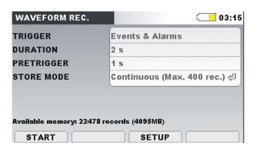
Figure 59: Waveform recorder capture screen
