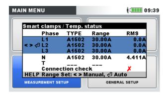
Figure 133: Automatically recognised clamps status
