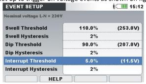
Figure 173: Waveform recorder setup for triggering on voltage events
