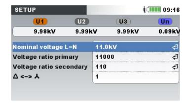
Figure 122: Voltage ratio for 11 kV / 110 transformer example
