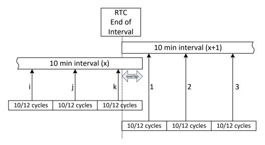
Figure 165: Synchronization and aggregation of 10/12 cycle intervals
