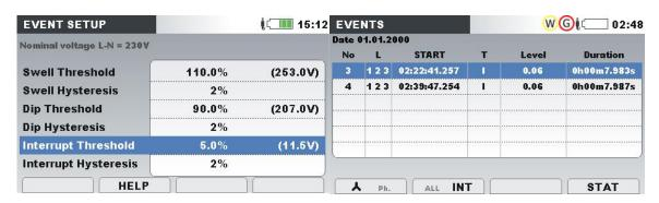
Figure 163: Voltage interrupts related screens on the instrument
