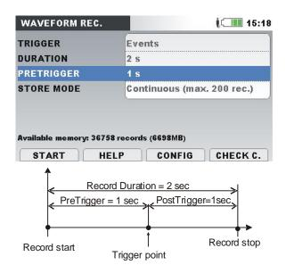
Figure 169: Triggering and pre-triggering description
