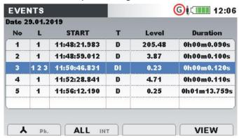
Shows poly-phase voltage interrupts only, according to the IEC 61000-4-30 requirements. START time and Duration in table is referenced to voltage interrupt only.
