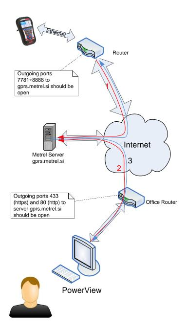
Figure 135: Schematic view on the remote measurements
