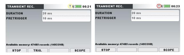
Figure 65: Transient recorder capture screen (waiting phase/recording) – MI 2893
