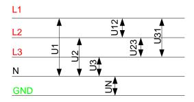
Figure 150: Phase and Phase-to-phase voltage
