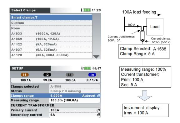
Figure 130: Current clamps selection for indirect current measurement
