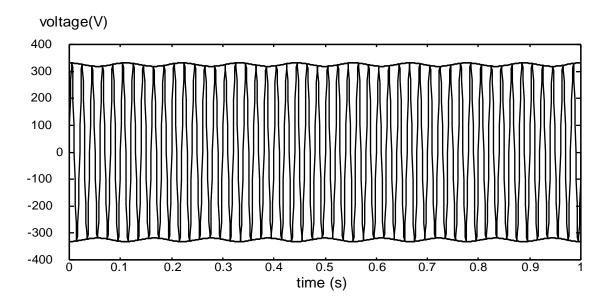
Figure 159: Voltage fluctuation
