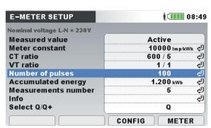
Figure 79: E-Meter Recorder setup menu
