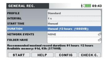
Figure 180: General Recorder setup to allow auto-recording restart, when reaches maximum file length
