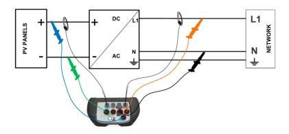
Figure 119: Single – phase inverter system
