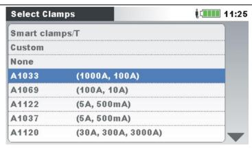
**Note:** For Smart clamps (A 1502, A 1227, A 1281, ...) always select "Smart clamps". Check in the Metrel General Catalogue, which clamps are developed as "Smart clamps).
