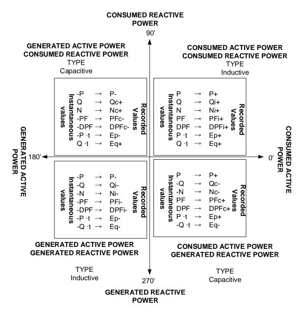
Figure 167: Consumed/generated and inductive/capacitive phase/polarity diagram
