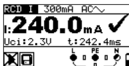
Figure 5.23: Trip-out current measurement result example
