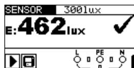
Figure 5.65: Example of illumination measurement result
