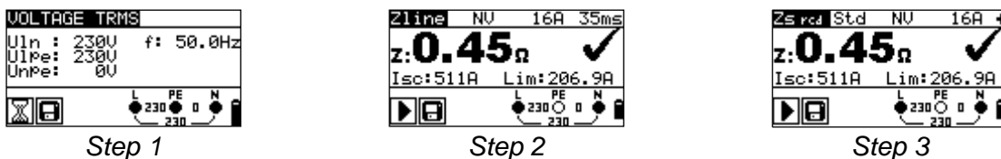
Figure 6.5: Individual steps of AUTO TT auto-sequence
