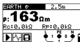
Figure 5.42: Example of specific earth resistance measurement result
