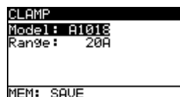
Figure 4.13: Configuration of current clamp measuring input
