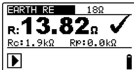
Figure 5.35: Example of earth resistance measurement result
