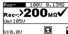
Figure 5.4: Examples of insulation resistance measurement result
