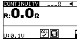
Figure 5.9: Example of continuous resistance measurement
