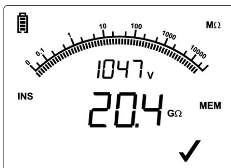
Figure 5.3: Example of insulation resistance measurement result
