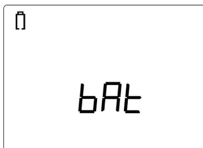
Figure 2.1: Discharged battery indication
