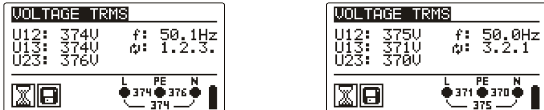
Figure 5.17: Examples of voltage measurement in three-phase system
