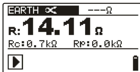
Figure 5.6: Example of selective earth resistance measurement results
