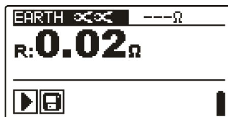
Figure 5.8: Example of contactless earthing resistance measurement result
