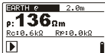
Figure 5.10: Example of specific earth resistance measurement result
