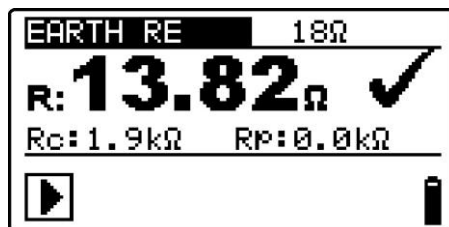
Figure 5.4: Example of earth resistance measurement result
