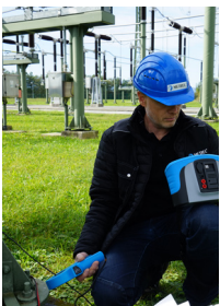
Flex or iron Clamps measures selective current from riser to grid.
