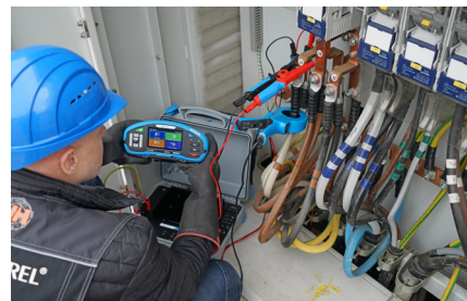
Iron Clamps connected to an external output to eliminate parallel resistances and current paths where several circuits are connected to live network.
