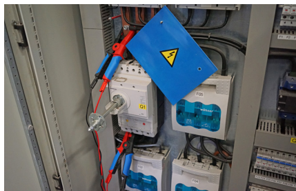
Four-wire type of connection with separated test crocodiles to eliminate serial resistances and bad connections. Test leads compensation is not needed.
