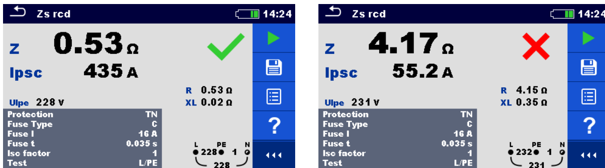
Figure 7.38: Examples of Zs rcd measurement result
