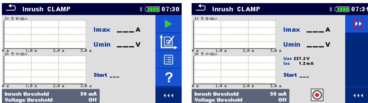
Figure 7.138: Inrush CLAMP menu – setup on the left, waiting for trigger on the right
