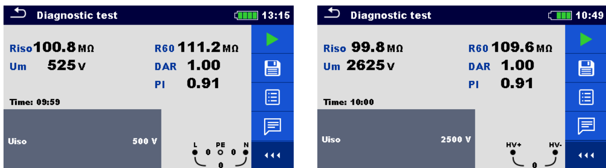
Figure 7.14: Examples of Diagnostic test result
