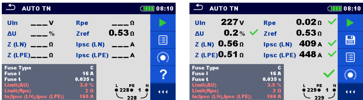
Figure 7.101: Examples of AUTO TN measurement results
