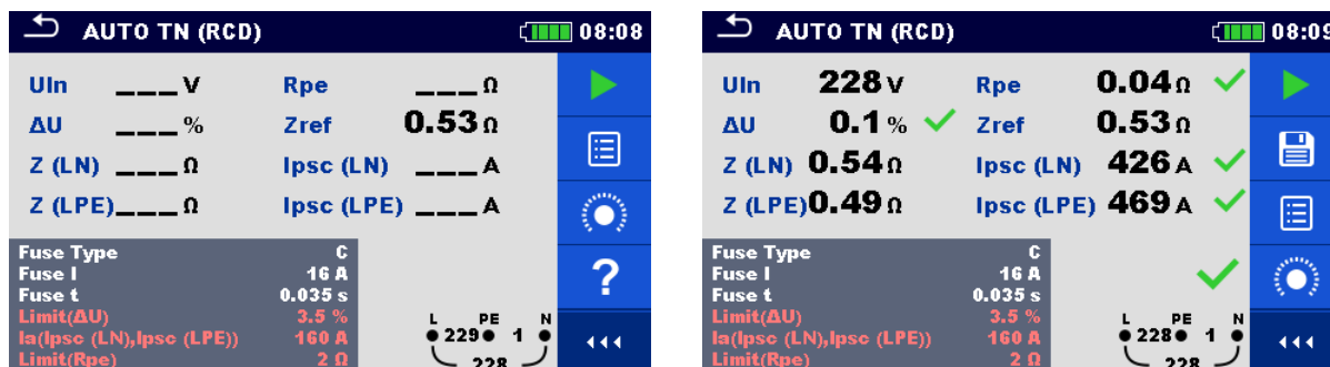
Figure 7.98: Examples of AUTO TN (RCD) measurement results
