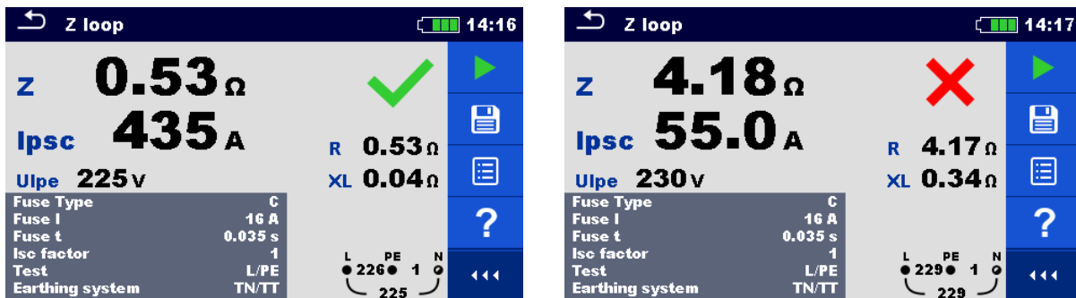
Figure 7.35: Examples of Loop impedance measurement result
