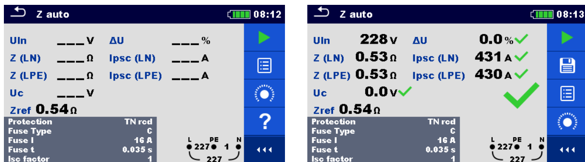
Figure 7.107: Example of Z auto measurement results
