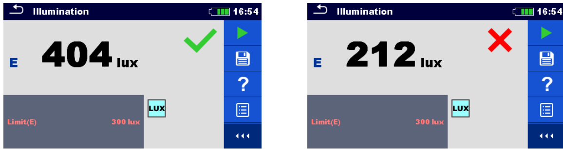
Figure 7.92: Examples of Illumination measurement result
