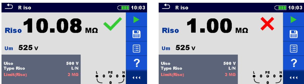
Figure 7.9: Examples of Insulation resistance measurement result
