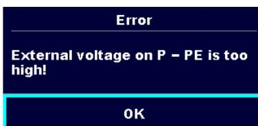
In pre-test a too high external voltage was detected between P and PE terminals. The measurement was cancelled.
