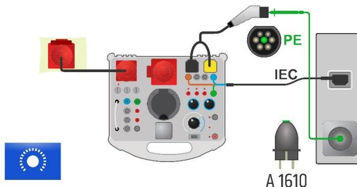
Compensation of IEC plug adapter resistance procedure
