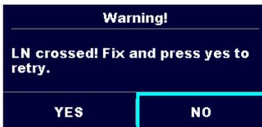
Warning for proper connection in some PRCD measurements. Connection of PRCD's plug must be changed in order to proceed.
