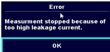
The measured leakage current was higher than 20 mA. Measurement was aborted.
