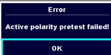
The polarity pre-test of the cable / PRCD has failed.
