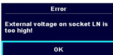
In pre-test a too high external voltage was detected between LN and PE terminals. The measurement was cancelled.
