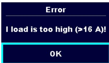
The load current higher than 16 A is detected. Measurement is aborted.
