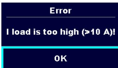
The average load current higher than 10 A over the last 5 min test interval is detected. Measurement is stopped. Recovery period for cooling is required before proceeding with tests!
