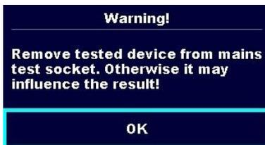
In 2<sup>nd</sup> step of Itou+Ifi test the DUT should be disconnected from mains test socket. Disconnect DUT from mains test socket and press OK to continue.
