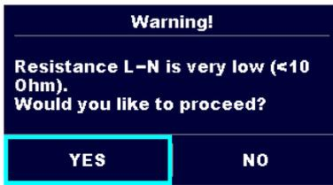
result in a high current after applying power to the device under test. If the too high current is only of short duration (caused by a short inrush current) the test can be performed otherwise not.
