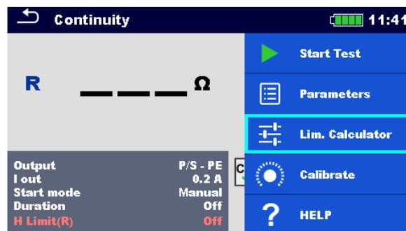
Limit calculator is a tool for determining the resistance high limit.
