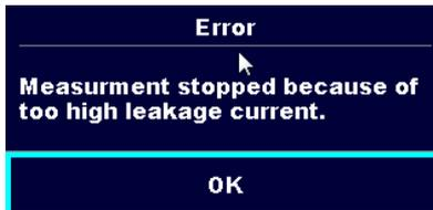
The measured leakage (Idiff, Ipe, Itouch, ...) current was higher than 20 mA. Measurement was aborted. Press OK to continue.
