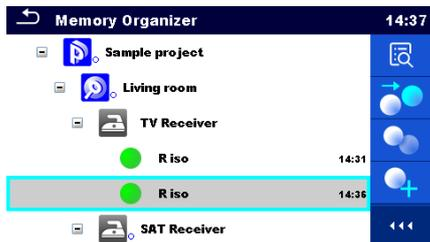
Retested measurement is saved under same structure item as original one.
