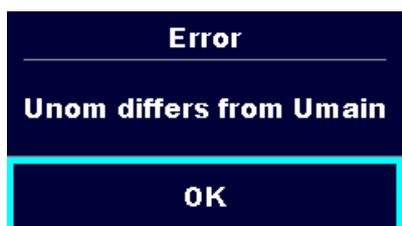
The set  $U_{nom}$  differs too much from the measured mains voltage. Parameter or mains voltage must be changed.
